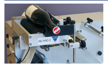
The half-automatic labelling machine for wrap-around-labelling of bottles and cylindrical objects.
