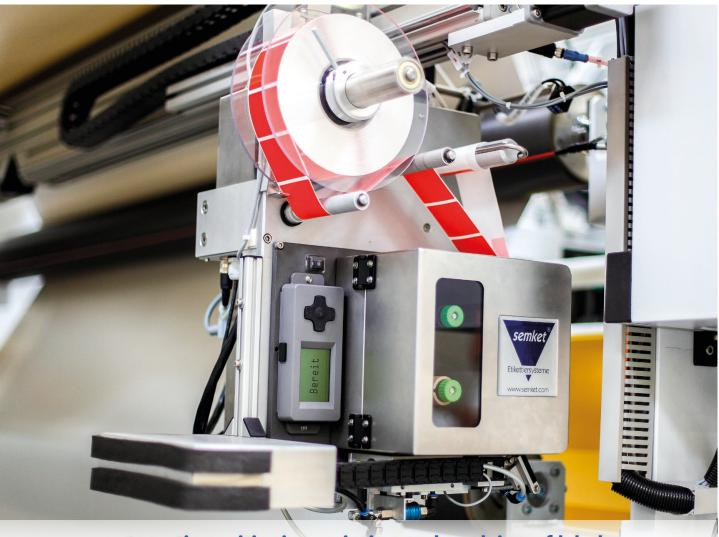
automatic positioning, printing and applying of labels
